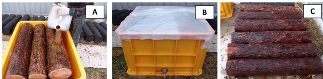
**Fig. 3.** Wood vinegar-treatment process: applying the wood vinegar on the longitudinal surface and transverse of the log (A), immersion for two weeks (B), and air-drying process (C)
