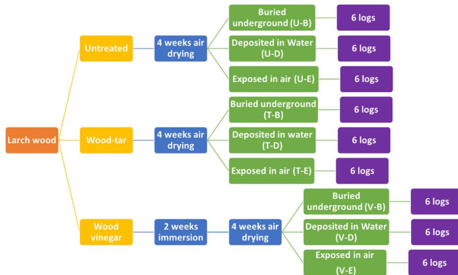
**Fig. 1.** The preservation treatments and durability test performed in the present study
