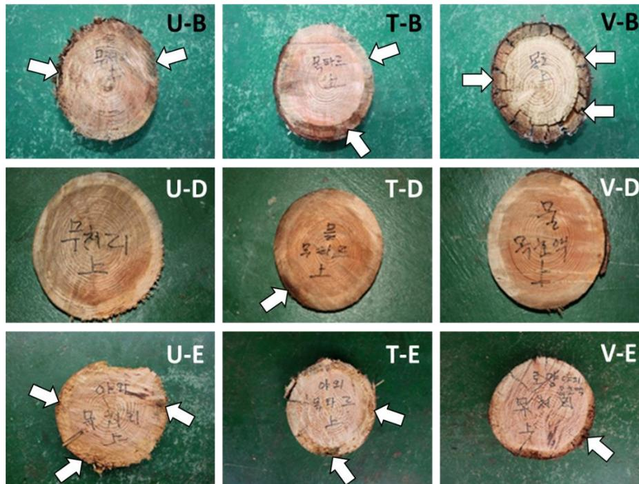
**Fig. 6.** The appearance of untreated (U-B, U-D, and U-E), wood tar-treated (T-B, T-D, and T-E), and wood vinegar-treated samples (V-B, V-D, and V-E) was examined after being buried in soil (U-B, T-B, and V-B), submerged in water (U-D, T-D, and V-D), and exposed to air (U-E, T-E, and V-E) for 53 months. White arrows indicate the degradation in the sapwood.
