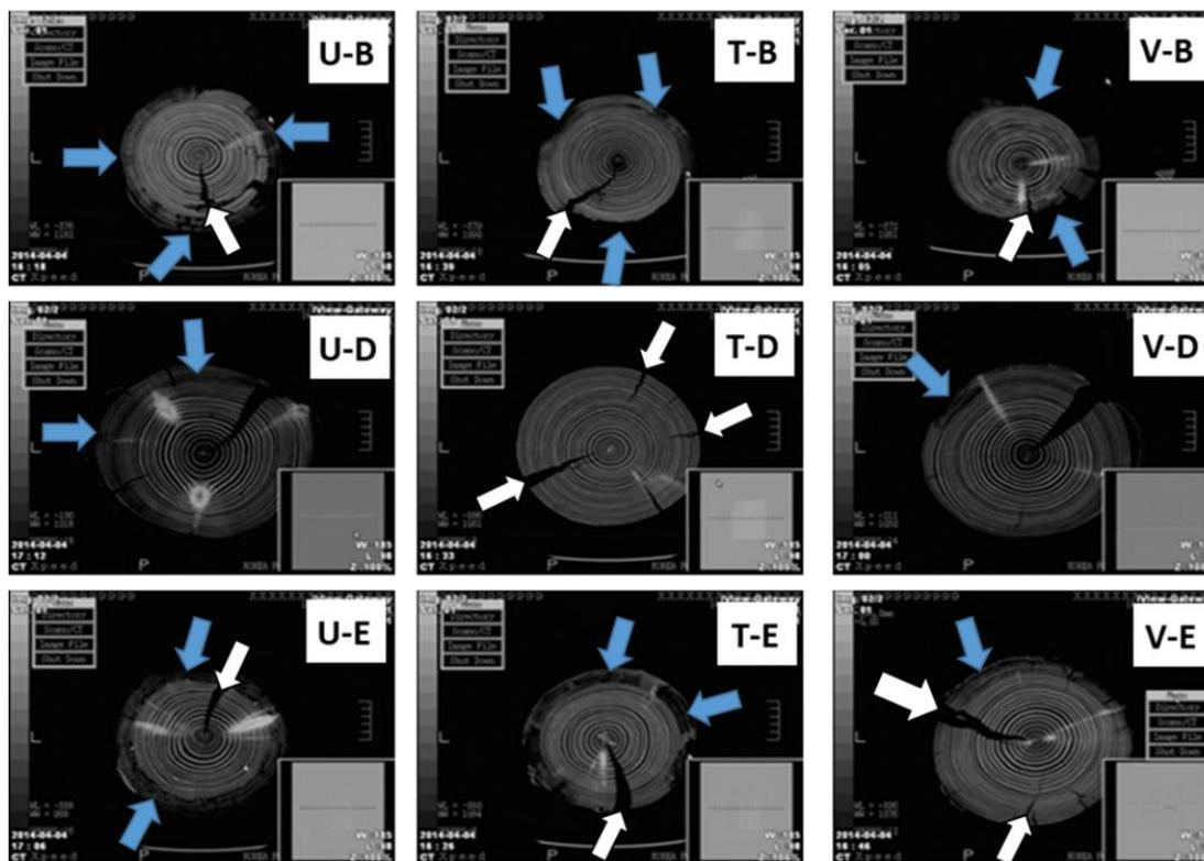
**Fig. 8.** CT images of untreated (U-B, U-D, and U-E), wood tar-treated (T-B, T-D, and T-E), and wood vinegar-treated samples (V-B, V-D, and V-E) that were examined after being buried in soil (U-B, T-B, and V-B), submerged in water (U-D, T-D, and V-D), and exposed to air (U-E, T-E, and V-E) for 53 months
