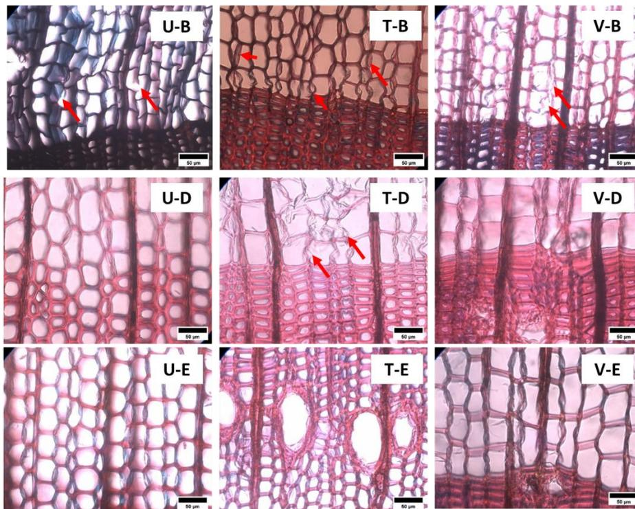
**Fig. 7.** Optical micrographs of untreated (U-B, U-D, and U-E), wood tar-treated (T-B, T-D, and T-E), and wood vinegar-treated samples (V-B, V-D, and V-E) of larch wood after being buried in the soil (U-B, T-B, and V-B), submerged in water (U-D, T-D, and V-D), and exposed to air (U-E, T-E, and V-E); Scale bars: 50  $\mu\text{m}$
