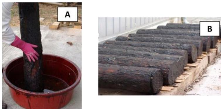
**Fig. 2.** Wood tar-treatment process: applying the wood tar on the longitudinal surface and transverse of the log (A) and air-drying process (B)
