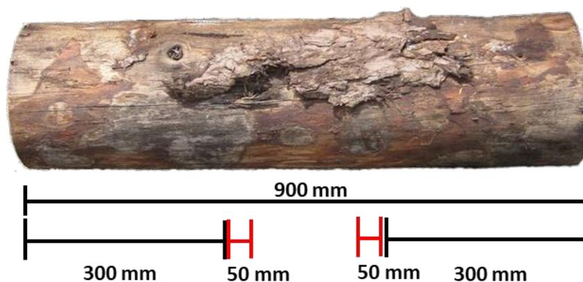
**Fig. 5.** The sampling position of the wood discs
