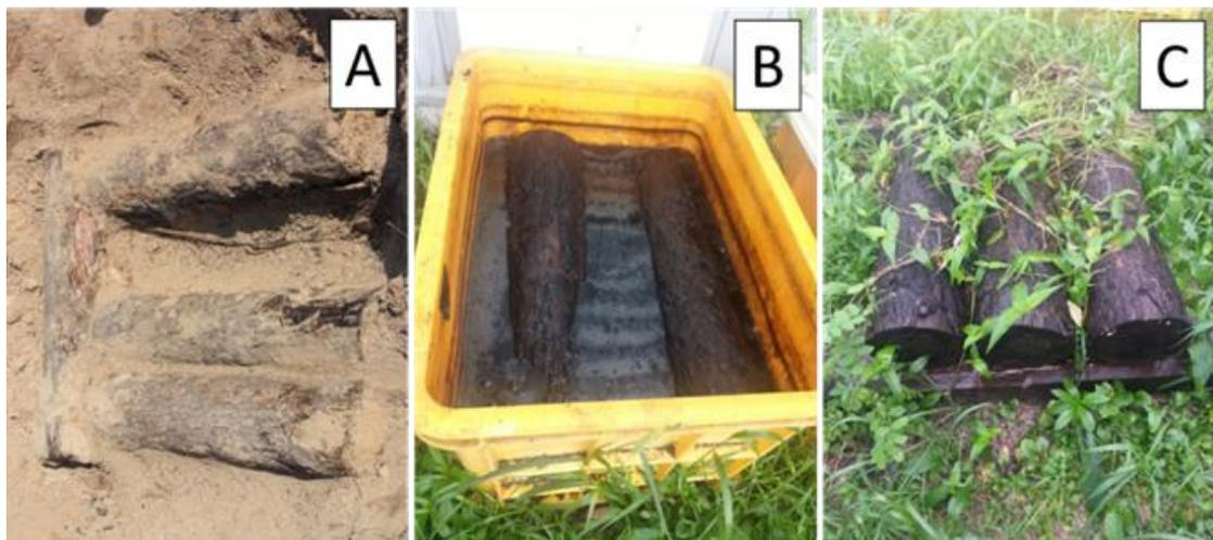
**Fig. 4.** The samples were buried in soil (A), submerged in water (B), and exposed to outdoor conditions, (C) for 53 months
