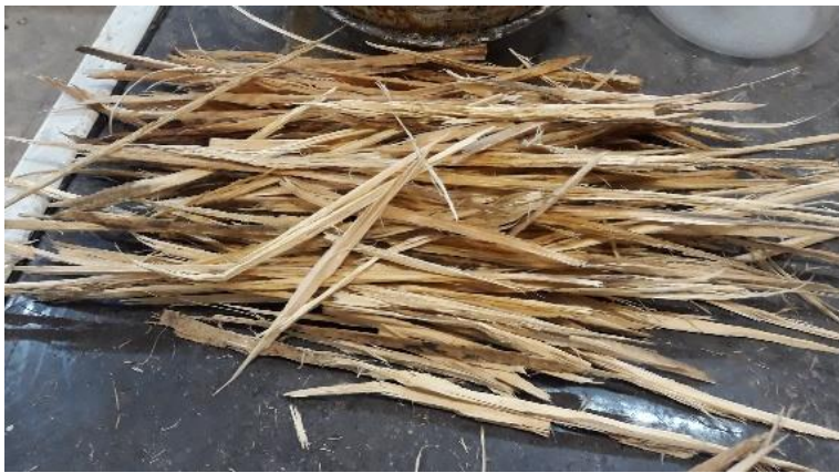
Fig. 2. Scrim strands produced from hydrothermally treated wood
