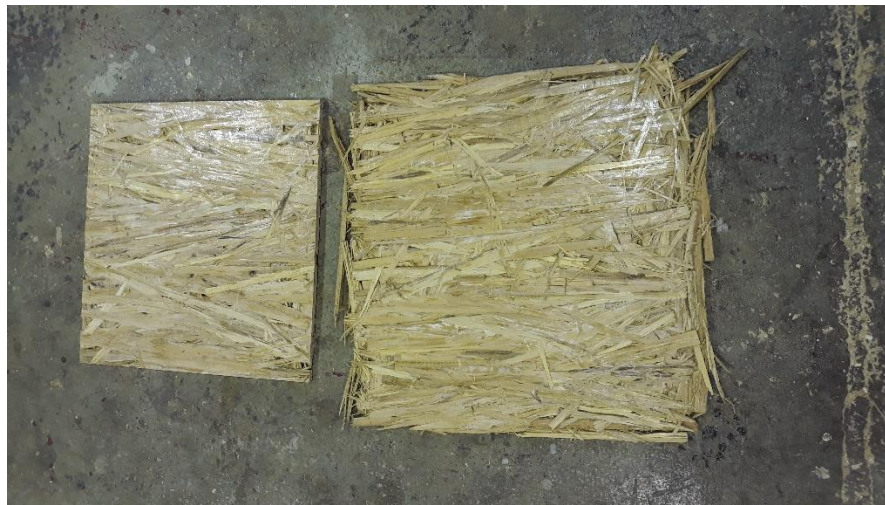
Fig. 3. A general view of manufactured scrimber composites before and after trimming
