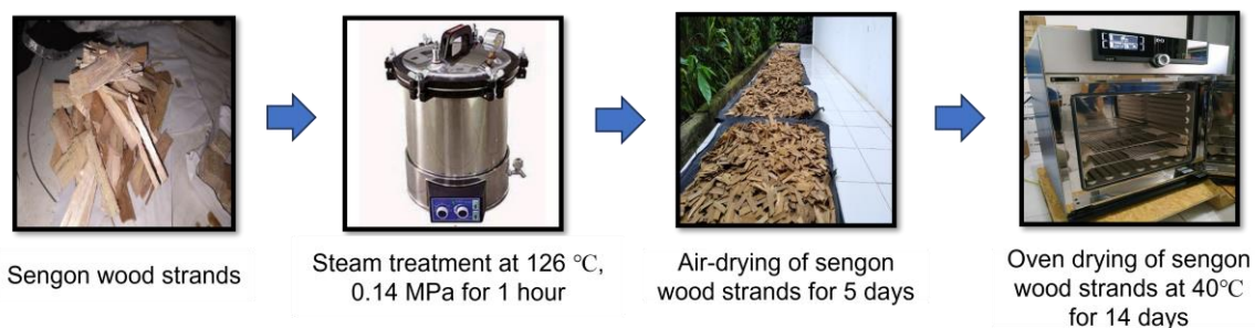
Fig. 1. Flowchart of sengon wood strands preparation
