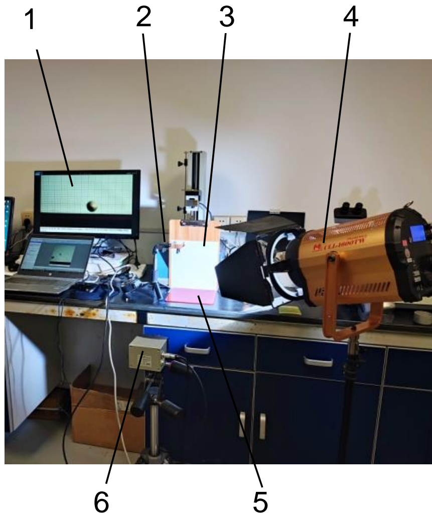
Fig. 3. Drop impact test. 1: Display; 2: Drop frame; 3: Background plate; 4: Light source; 5: Base plate; 6: High-speed camera
