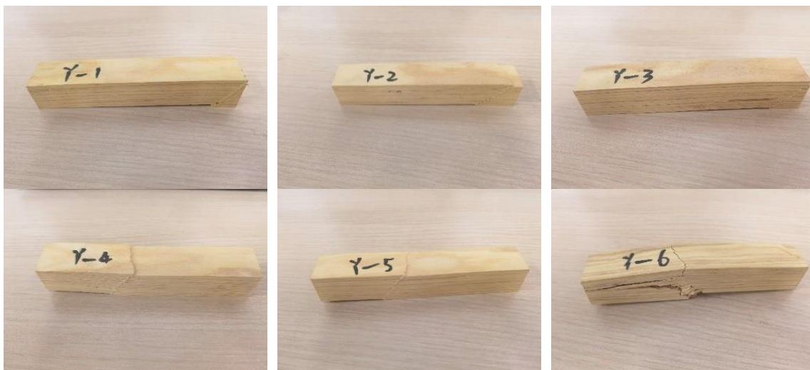
Fig. 12. Compression failure morphology of the specimen
