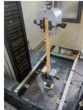
b. Specimen L-2-3 is used for tensile test
