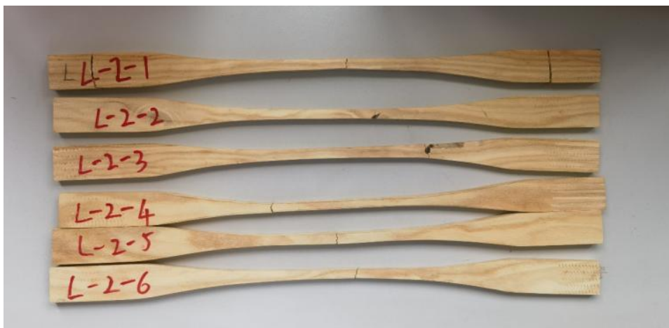
Fig. 10. Failure morphology of tensile specimens
