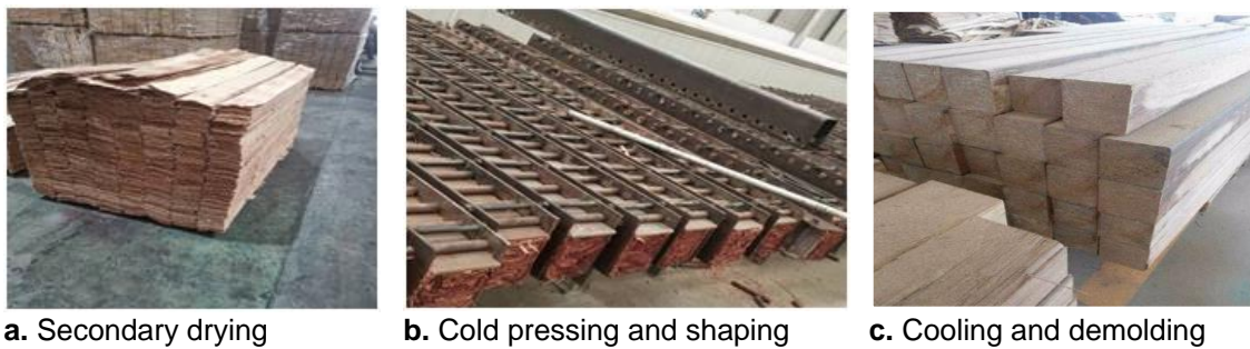
Fig. 1. The main production process site of ginkgo scrimber
