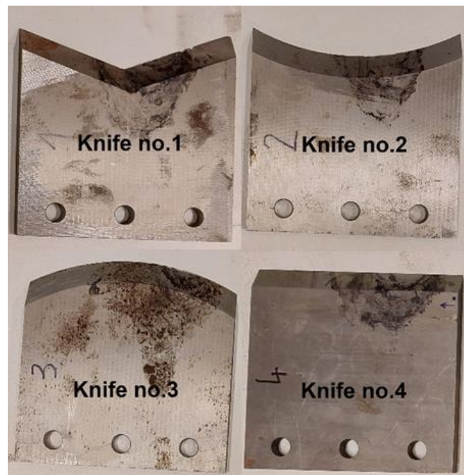
Fig. 4. Cutting knives with different cutting edges
