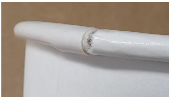
Fig. 11. The rim roll of the cup has split near the side seam, exposing the fiber structure of the paperboard
