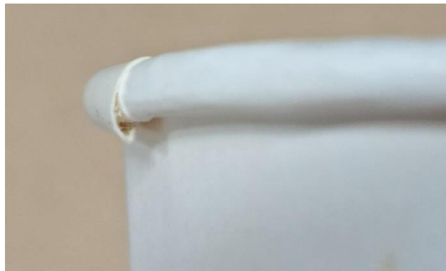
Fig. 13. Delaminated rim roll with exposed fibers
