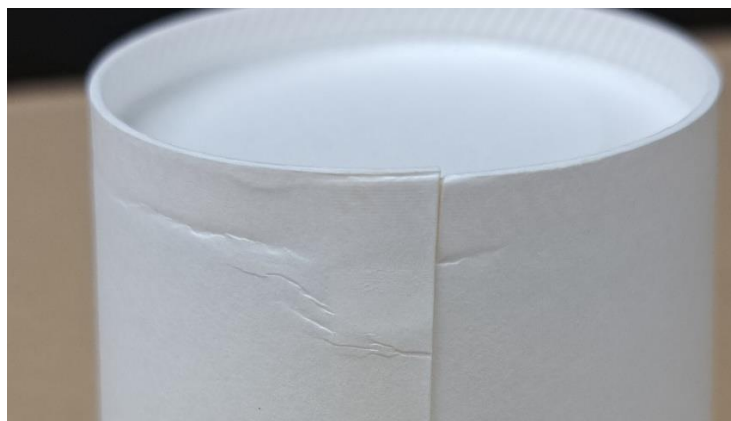
Fig. 16. Buckling of the side seam area near the bottom
