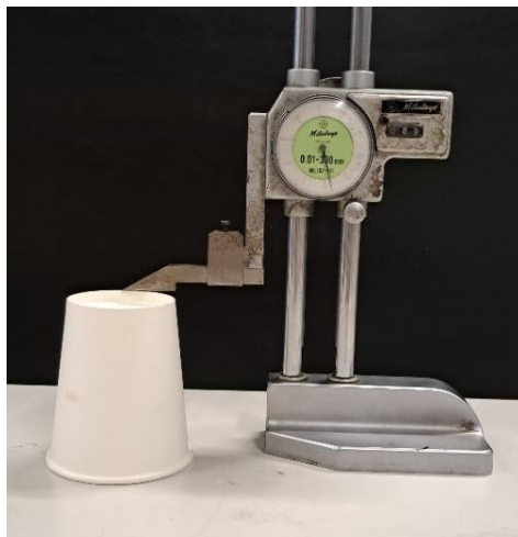
Fig. 6. The device that was used to measure cup height
