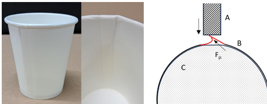
Fig. 14. Cup with a majorly buckled side seam (Material 1) and suspected mechanics of defect formation. A: Sealing tool, B: Wall blank, and C: Mandrel
