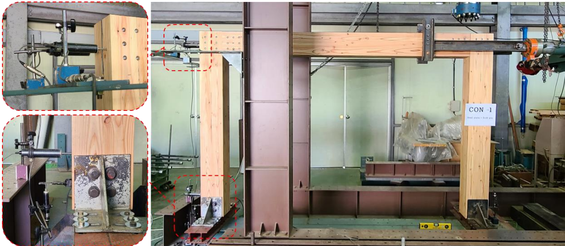
Fig. 4. Test setup for laminated timber portal frames
