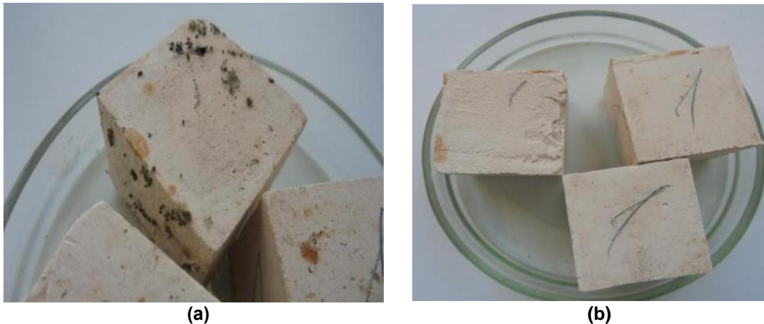
Fig. 1. Visual shape of the samples after the test: (a) - control sample, (b) - sample modified with R. sachalinensis extract
