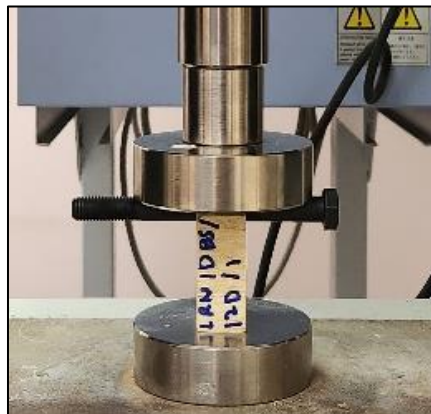
Fig. 1. Test set-up for bolt bearing strength test
