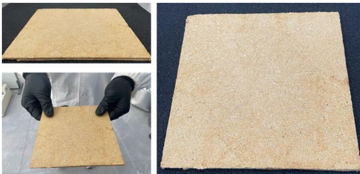
Fig. 2. Surface morphology of straw fiberboard (CLS)
