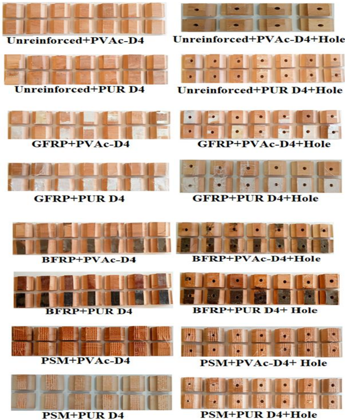
Fig. 8. Failure modes of the unreinforced and reinforced with FRP samples
