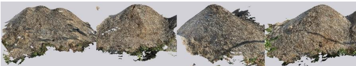
Fig. 5. LiDAR scans of piles in the 3d Scanner App performed by iPhone 14 Pro Max
