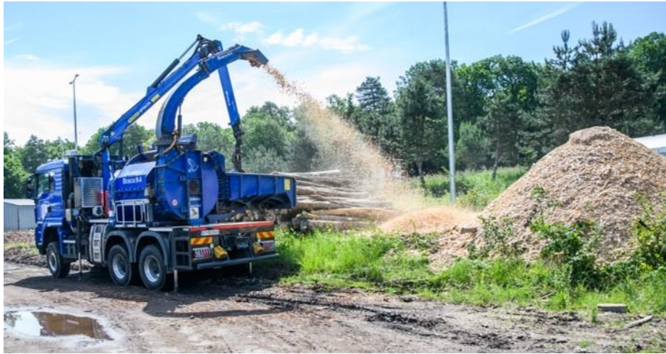
Fig. 2. Preparation of the experimental piles with chipper
