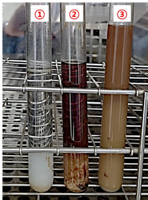
Fig. 3. Dispersion state of flame-retardant in wax solution according to ball milling processing time (① prior to ball milling, ② 24 h post-ball milling ③ 36 h post-ball milling)
