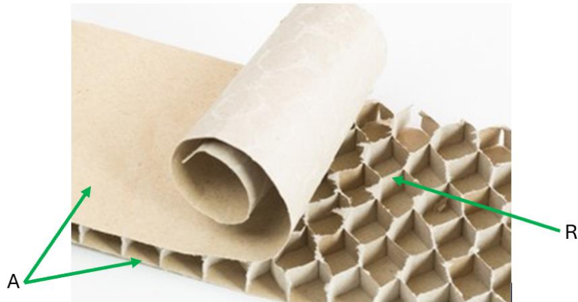
Fig. 1. Construction of honeycomb paperboard: A, flat layers of paperboard, R, paperboard core
