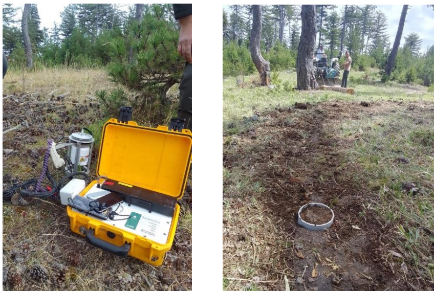
Fig. 4. LI-8100 LICOR was used to measure soil respiration on the skidding trail
