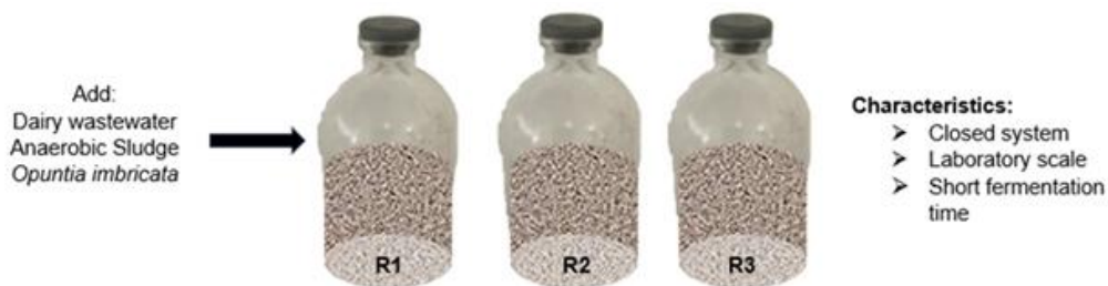
Fig. 2. Schematic design of batch reactors (triplicate)
