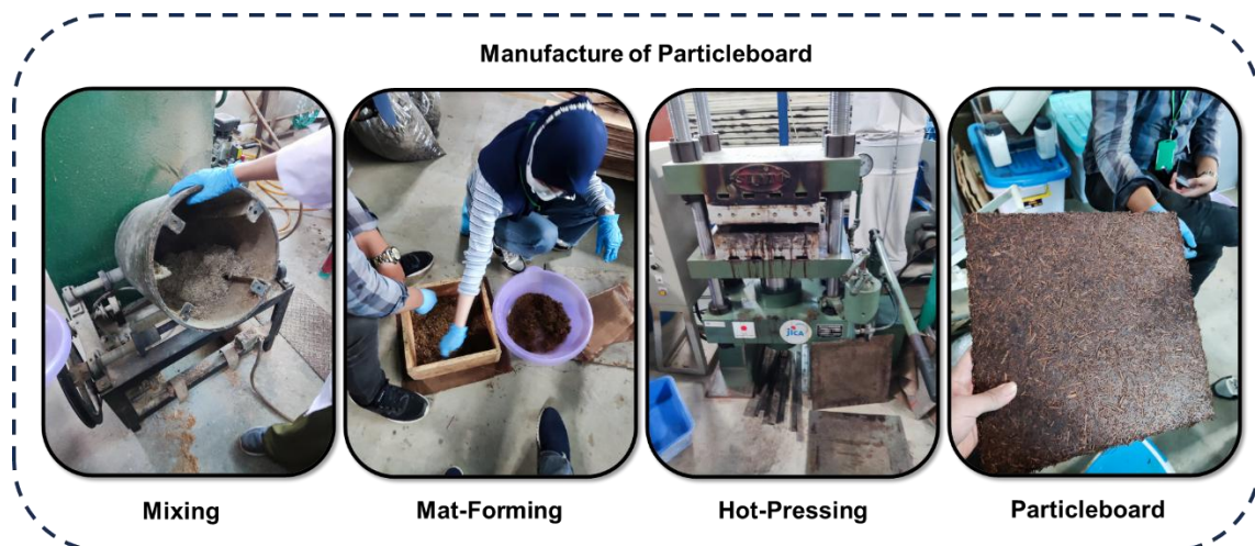
Fig. 2. Manufacturing of particleboard
