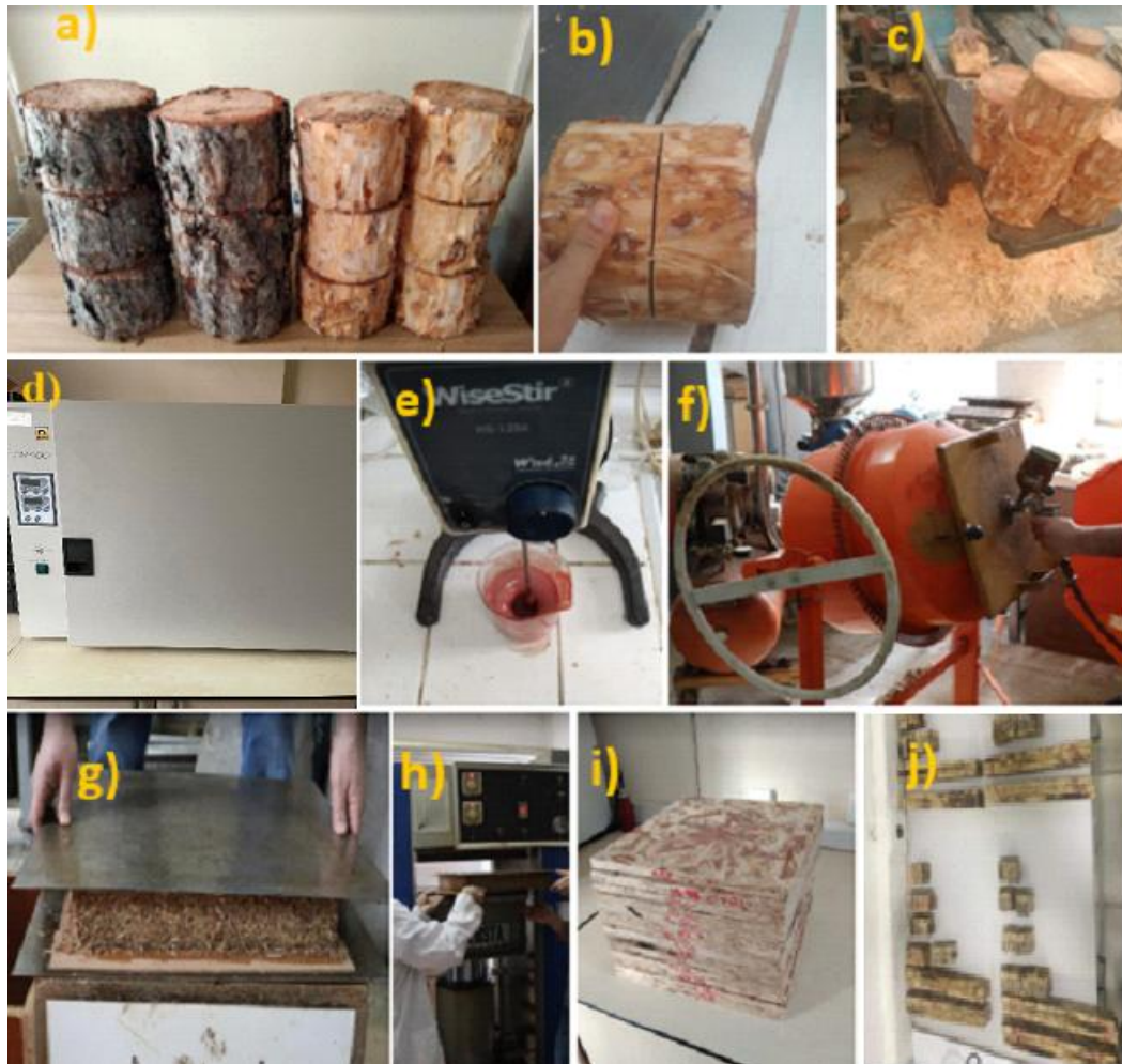
Fig. 1. PB manufacturing process: a) Wood sample, b) notch on wood, c) wood chipping, d) drying, e) glue preparation, f) gluing, g) mat forming and cold press, h) hot press, i) produced PB, and j) test samples
