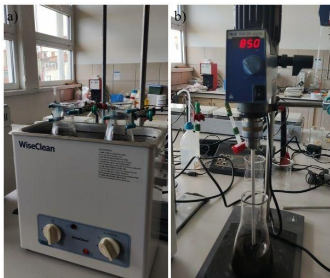
Fig. 1. The preparation of coatings: a) ultrasonic bath, b) mechanical mixer
