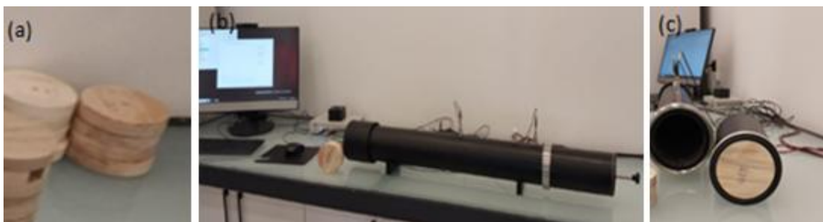
Fig. 1. a) Test specimens, b) impedance tube, c) impedance tube with specimen attached
