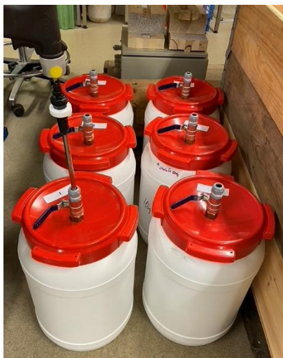
Fig. 2. The containers and gas probe used for the off-gassing tests
