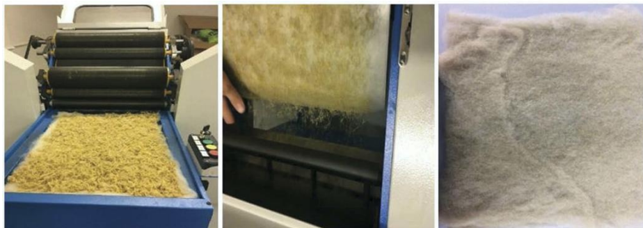
Fig. 3. Laboratory-type carding machine and carding band made of broomcorn stalk fibers
