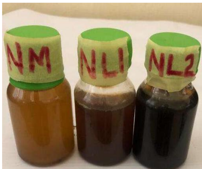
Fig. 2. Different color change indicating neem leaf extract (NM), neem leaf extract with \text{AgNO}_3 after 1.0 h (NL1), and after 6 h (NL2)
