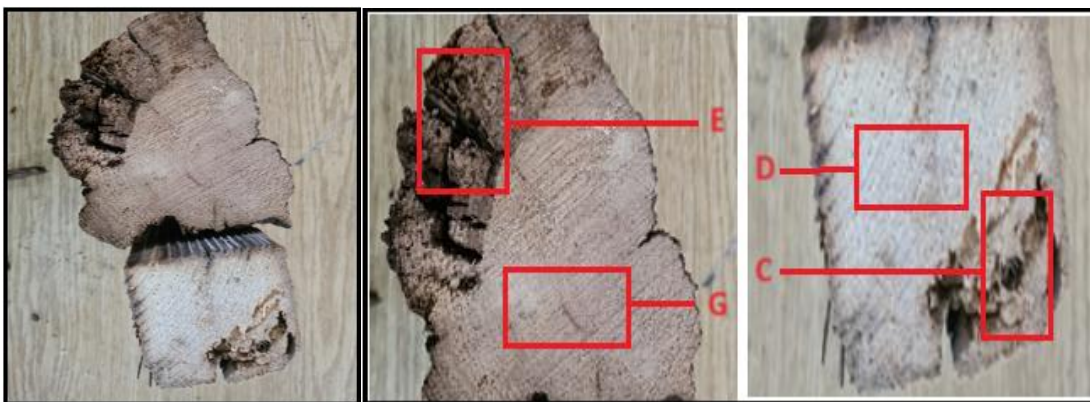
Fig. 3. The analysis sections (internal - external) of the wooden samples (E, G, C, D)
