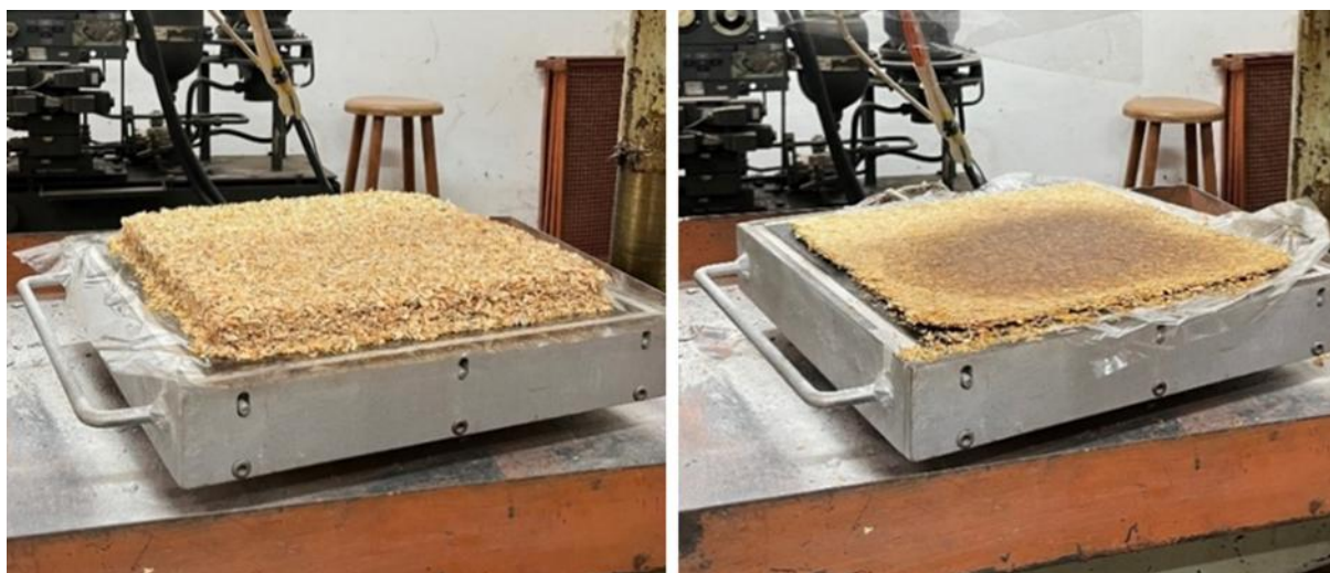
Fig. 2. Pressing stages: Pre-pressing (a); and post-pressing (b)
