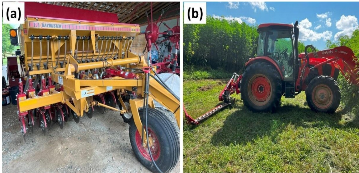
Fig. 5. (a) Seed drill equipment for spacing the seeds and (b) sickle bar mower for harvesting industrial hemp plants
