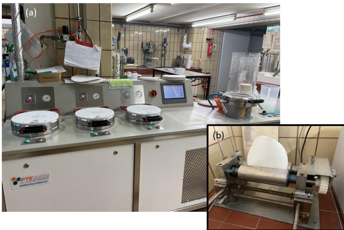
Fig. 1. (a) Rapid-Köthen Automatic Sheet Former; (b) Rolling machine at PMV, TU Darmstadt
