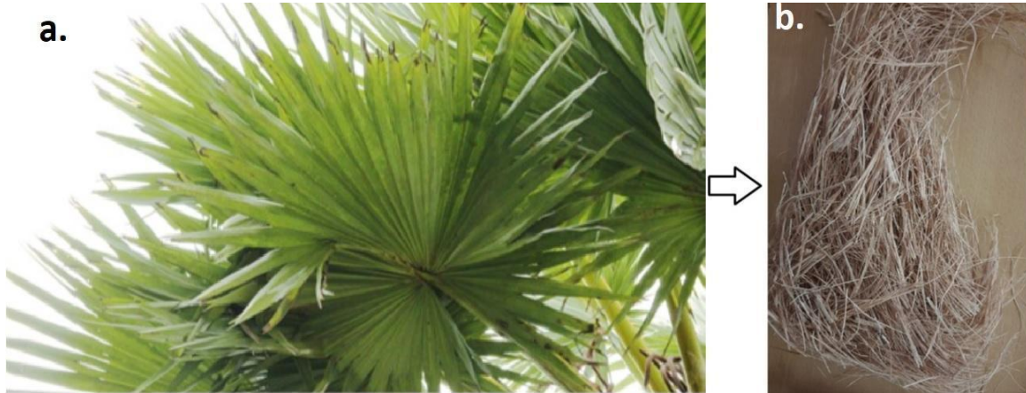
Fig. 1. (a) Leaves of palmyra palm ( Borassus flabellifer ); (b) Extracted leaf fibers
