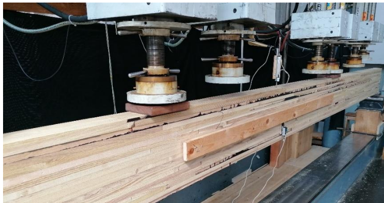
Fig. 5. Test set-up of the full-scale bending tests with Robinia glulam (Schenk 8piston/200kN, Darmstadt, Germany)
