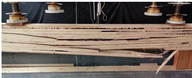
Fig. 6. Typical fracture pattern of a Robinia glulam beam after failure
