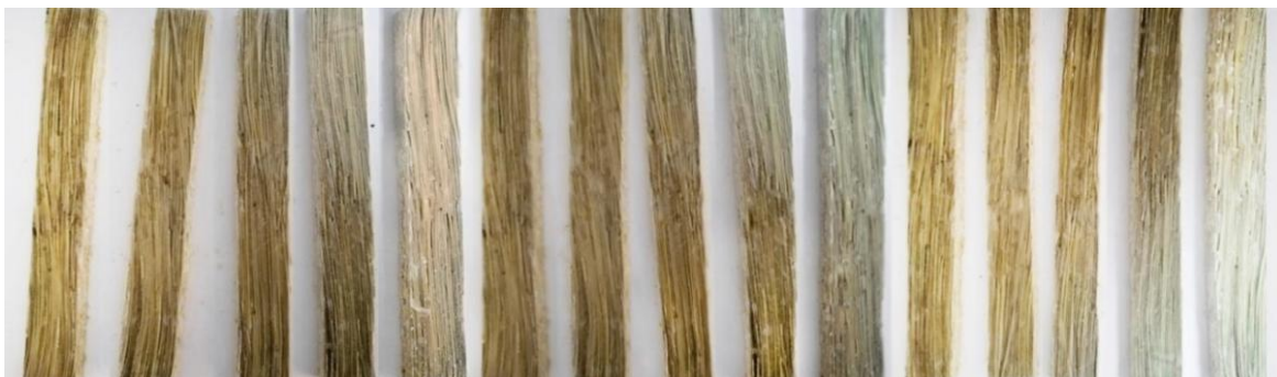
Fig. 3. An example with 15 samples from a plate with HE40 resin used for the tensile test
