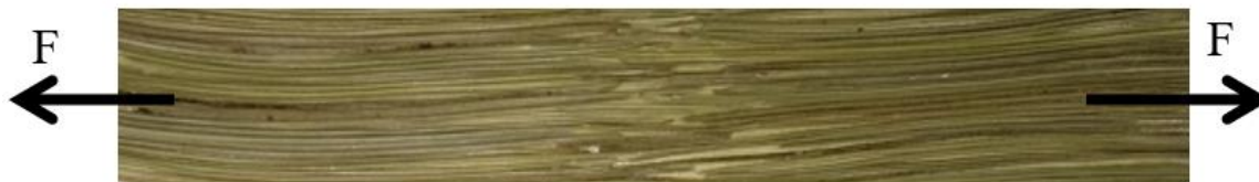
Fig. 4. An example of how the tensile test force was applied along the fibers
