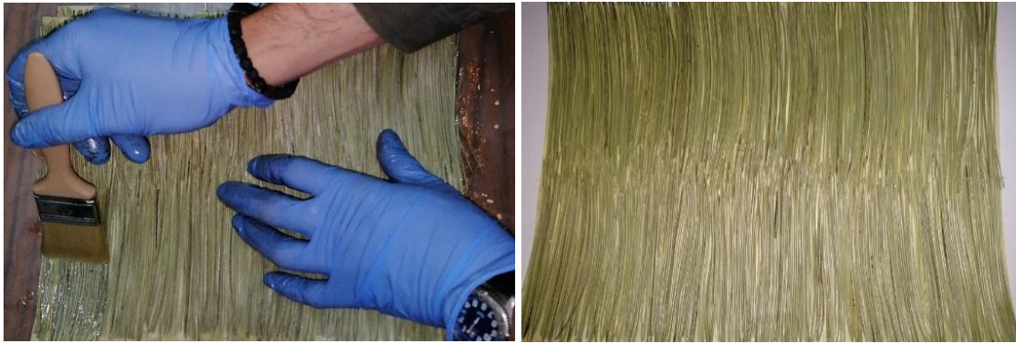
Fig. 1. A detail with the final shape of a lamella with pine needles placed on a paper waste support
