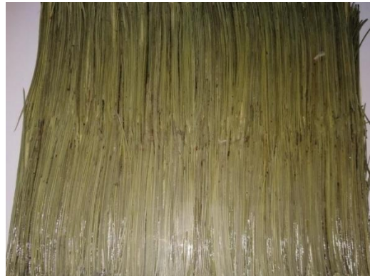
Fig. 2. An example of a plate with HE40 resin reinforced with pine needles trash and paper waste
