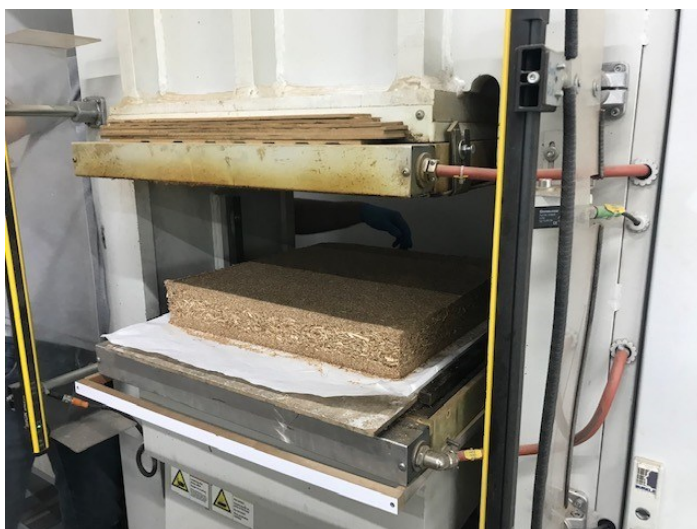
Fig. 4. Pressing of chip drafts (Bürkle press)
