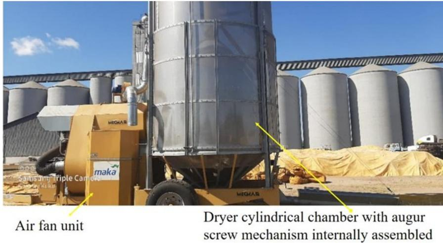
**Fig. 5.** Portable dryer
