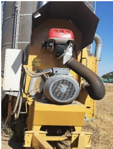
**Fig. 8.** The fan and burner assembly unit
